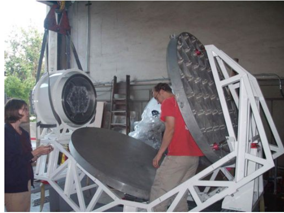
Figure 2-1: a : Schematic of the QUIET instrument, showing the electronics enclosure, cryostat, and mirrors. A view of the inside of the cryostat is shown as well, detailing the feedhorns, OMTs and polarimeter modules. b : Photograph of the cryostat (the top section had been removed for a measurement when the photograph was taken, allowing a view of the hexagonal array of feedhorns) and mirrors.
