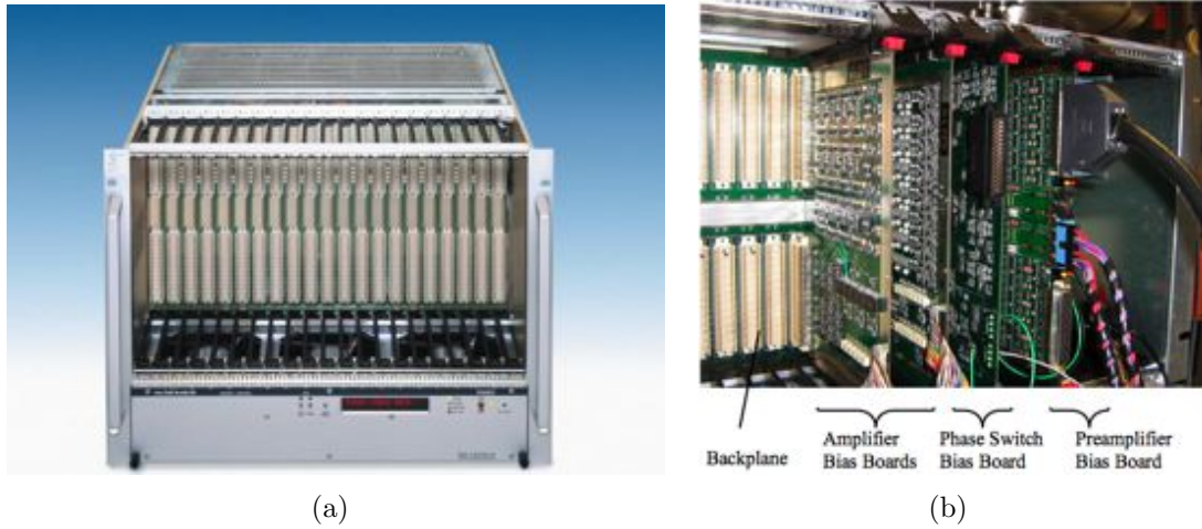
Figure 2-30: a : Manufacturer's picture of the Weiner crate and backplane ( http://www.wiener-d.com/index2.php ). This houses the ADC cards, crate computer, and timing cards for QUIET. b : A photograph of the backplane, populated with two amplifier bias cards, a phase switch bias card, and a preamplifier bias board.
