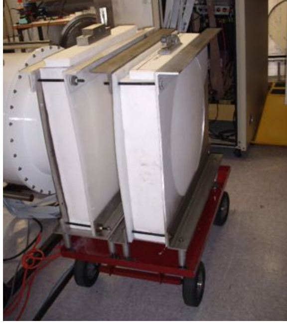
Figure 3-5: Two zotefoam cryogen buckets, supported by adjustable feet above a cart, which allows them to sit at the appropriate height for the receiver to see directly into the absorber insert. The cart allowed us to easily and quickly change between the two cryogenic loads for the Y-factor measurements. Measurements were performed such that we wheeled one load in front of the cryostat, integrated over 10 seconds to obtain the average power (voltage) for a given load, wheeled the cart out of the beam and rotated it such that the second load could be aligned with the beam. Each load weighs \mathcal{O}(100 \text{ lbs}) .
