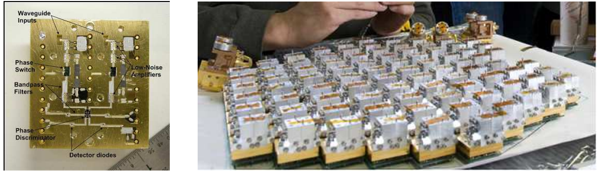
Figure 1: A 95-GHz module with the radiometric components integrated (left) and the 90-element 95-GHz array under assembly (right).
