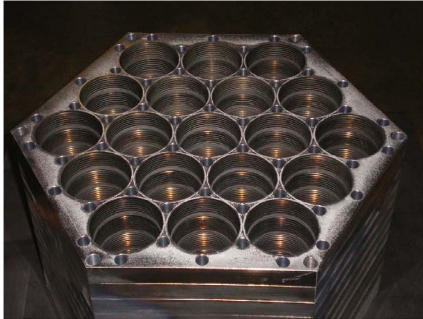
Figure 2.2: Top-view picture of the Q-band platelet array, which is composed of 19 feedhorns. All the polarimeter modules are attached at the other side with septum polarizers.
