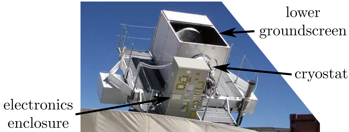
Figure 4.8: Photograph of QUIET, with the lower groundscreen indicated. Also labeled are the electronics enclosure and the cryostat (which is mostly obscured by the enclosure).
