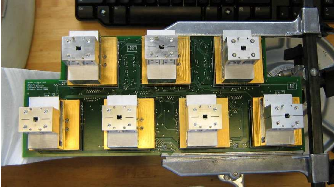
Figure 4.2: Photograph of seven Q-band modules, with septum polarizers attached, installed on an MAB. Photo credit: Ross Williamson.
