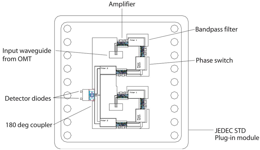
FIG 3.—Layout of polarimeter module in package. Placement of parts will be done by hand for small numbers, by automated equipment for large numbers.
