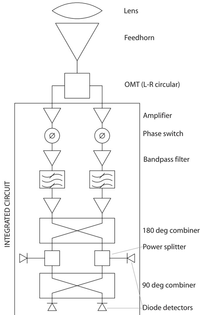
FIG 2.—Block diagram of a polarimeter that detects Stokes Q and U. A full array will be populated with such modules. In about 5% of the array, the OMT will be replaced with a hybrid coupler and a reference load to produce Stokes I.
